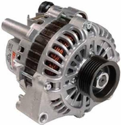
From the department of fixing things that are not broken, it seems that several vehicle manufacturers now use special variable-output alternators that are under control of temperature and engine management systems. No longer will you be able to simply pop a bonnet and check for around 14V at the battery terminals with the engine running as a simple measure of charging system integrity.
