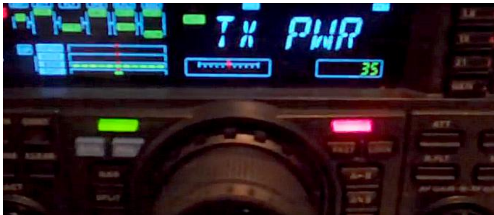
Using VFO-A to select TX Power mode and VFO-B to change the value
