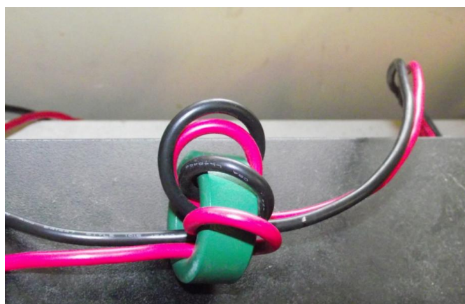
Ferrite ring on the power cable to stop RF feedback
