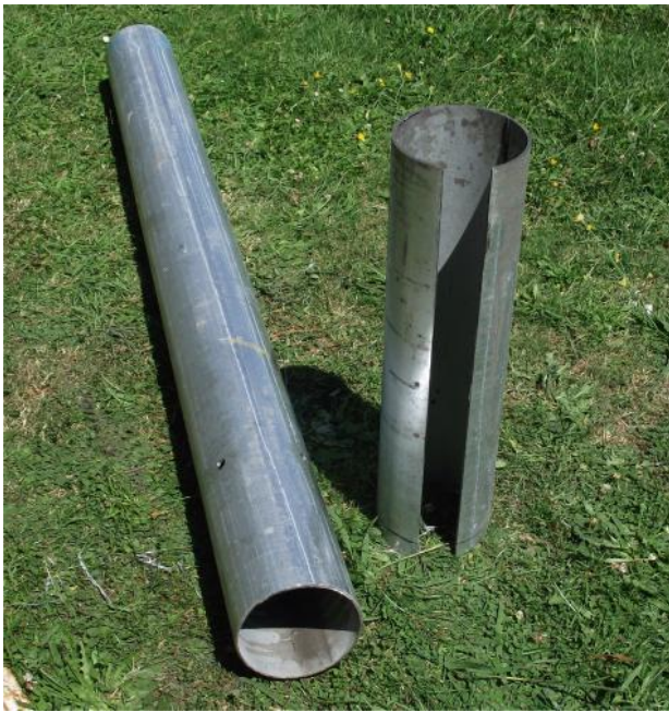
The pipe extension and the prepared sleeve
