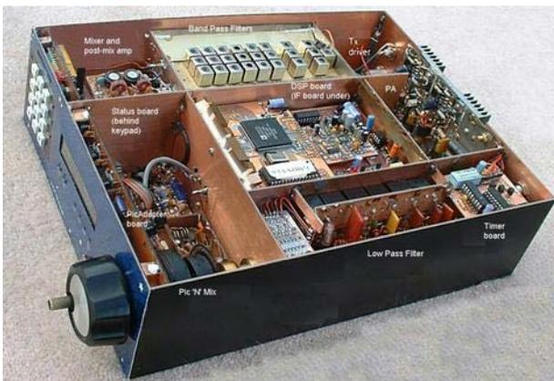
McDiarmid said the radio is as feature rich as some of the more expensive commercially available HF transmitters. He said it has been shown to be extremely effective at shielding from interference, a bane of HF transmissions. Details of the design and features are provided by Peter Rhodes in a 45-page PDF file at [www.tracey.org/wjt/temp/picastar-all.pdf](http://www.tracey.org/wjt/temp/picastar-all.pdf)
