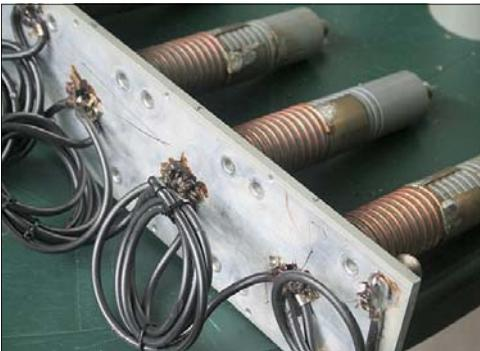
Bottom view, each resonator is connected via a capacitor to three lengths of coax. one in each adjacent section, the third being a quarter wave-length line.
