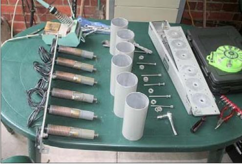
The duplexer almost completely stripped down. Unsoldering the helical resonators from their coax connections proved too hard, so I went for plan 'B' - only unsolder the troubled one.
