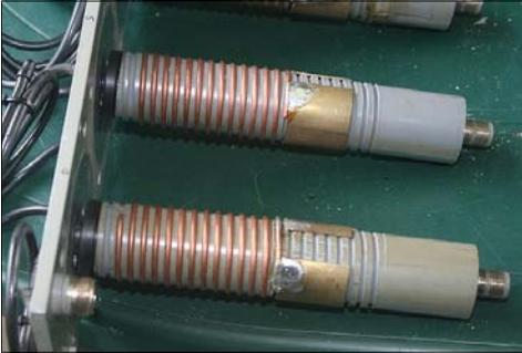
Two of the helical resonators, at 50MHz true cavities would be enormous.
