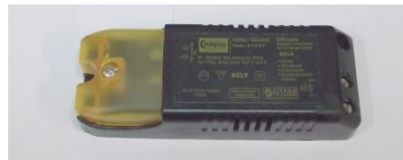
Typical Switch-mode converter
