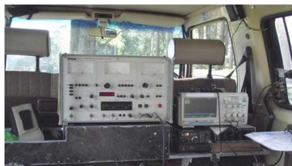
Using a VHF test set & Cro as a spectrum analyser for tracking the noise source
