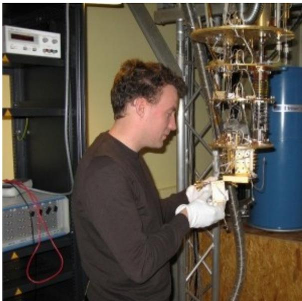
In the amp experiment the use of a single-electron pump, a device in which voltage pulses prompt electrons to quantum-mechanically tunnel across barriers one at a time is used. The researchers tracked the paths of individual electrons by detecting changes in the electrical charge stored at points between the barriers. Primitive electron pumps have existed since 1990, but this is the first time that changes in charge have been detected for each hop of an electron.
