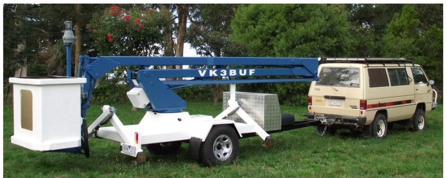
*The completed unit, shown with antenna rotator column*
