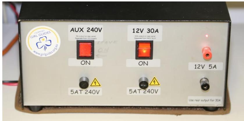
Now for some notes, You will notice that the front panel has two power switches, the first only turns on a pair of 240V sockets on the back panel, it has NO effect on the 12V output, and for the most part (for now) can be left turned off.
