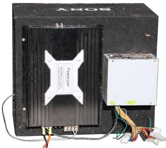
A 1KW speaker run by a 550W PC supply!
