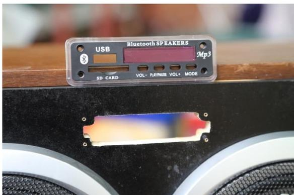
One of the first tasks was to cut a hole in the craft wood front panel, this was a bit tricky as the Chinese music player I had selected has some fairly fine dimensions between the circuit board and the very small mounting screw holes. If it were to be mounted in a plastic or metal panel the job would have been a lot easier, however careful persistence with some small files eventually paid off.
