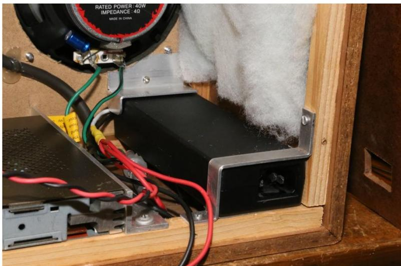
I looked through my junk box and ended up using a 7A switchmode power supply for 240V operation. I thought I had a 4A unit, a tad smaller, but that search ended badly.
