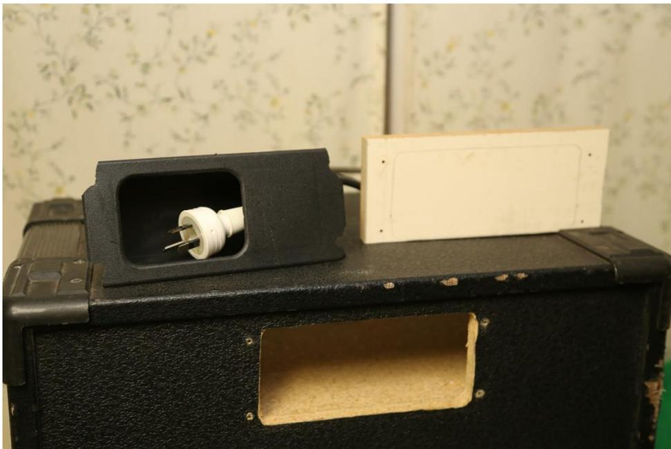
On the back of this unit was a plastic box intended to have the rolled up power cord stowed, however as it was starting to fall to bits, I converted it to use a detachable cord by fitting an IEC style socket to the back panel. The white block of wood atop the speaker was soon to be sprayed black, and have a socket fitted.
