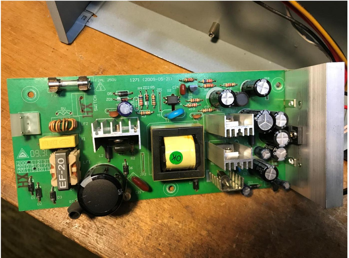
And here is the power supply, luckily easily extracted. The output cable to the main board had me a tad confused, it had two red wires, nothing unusual, a common trick done to lower the resistance & up the current, however my meter indicated that they were not connected to each other, unlike the two black wires.
