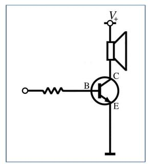
The simplest amplifier is a resistor feeding a single transistor. The Nano's output is limited to an absolute maximum of 30mA, ideally 20mA. An 8 ohm speaker on 5V will pull over 600mA, way more on 12V, (although I doubt you'd need that much audio from a practice oscillator), anyway that's way more than the Nano can handle on its own.
