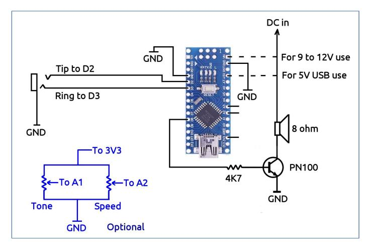
Here is the circuit, along with the optional pots. You can also add a second 4K7 resistor and transistor to pin 'D13' and use it to key a radio that does not have a paddle input.
