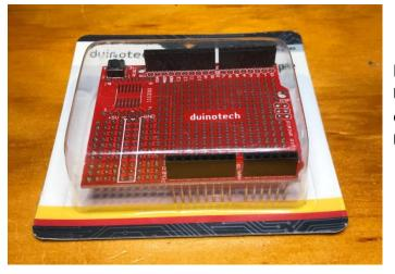
IF you would prefer using an Arduino Uno, then there are these plug in 'shields' as they call them, plenty of room for a transistor or two.
