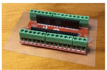
These screw terminal adapters are specifically made for the Arduino Nano, with the screw terminals labelled with their Arduino names.
