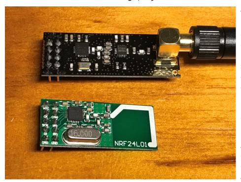
These NRF24L01 based units from Nordic Semiconductor come in two basic flavours; one with a built in circuit board antenna, and the slightly larger one that uses an SMA connector to attach an antenna, the latter also has an RF amplifier stage to up the power levels for extended range. (0 dBm)
