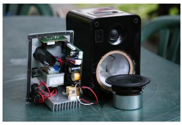
This month I was going to do a repair on a powered speaker I acquired, and say about some of the crazy choices made in its design, things like using a finned heatsink, good, but enclosing it inside a very small speaker box buried in a sheet of polyester speaker wadding, VERY bad.
