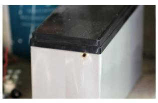
After replacing the so called 'battery charger' with a nice metal boxed switchmode, I later noticed a nasty acid smell, which lead to a very warm 7AH sealed lead-acid battery, that had a small hole burned into its end, a dead cell as evidenced by that battery quickly dropping to 11 volts after disconnection. No excuse for that plug pack charger wanting to call the fire brigade though.
