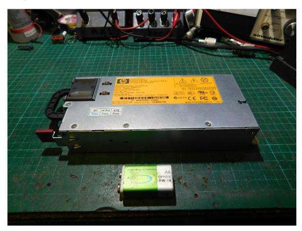
They duly arrived and the first test was to make sure they were working. After shorting 2 terminals I measured 12.3 volts on the output, and fitted a 55 Watt car headlight that worked fine, so far good enough. I then opened up the power supplies and started the modifications.
