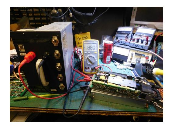
Upon initial tests with a decent load (Thanks for the loan of the test load AI) a squeal was heard from the supply when drawing over 10 amps.. It was discovered that the supply was trying to shut down on the over voltage safety. A quick adjustment of a second pot stopped the supply from trying to shut down and was as quiet as a mouse when loaded up to about 38 amps, the maximum the load could draw from the power supply.
