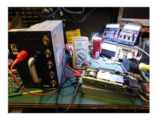
Out of curiosity I stoked up the spectrum analyser and had a look at the broadband noise being emitted from the supply from 10 KHz to 30 MHz, a very rudimentary test due to me just waving an antenna around the power supply under all loads. I did not have enough space on the bench to properly set up and test the EMI/EMC being radiated with my LISN (and the speccy set up in EMI/EMC mode). Below is the result with the antenna positioned at the "noisiest" part of the supply.
