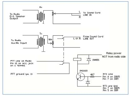
There will be a difference between the radio and the computer, the mic pre-amp will see and amplify this and send it on to be transmitted!
