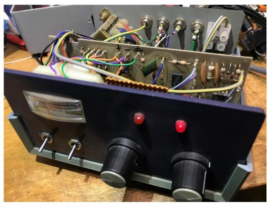
My main decoder was this ETI730, it worked extremely well and could resolve signals with a very narrow shift.
