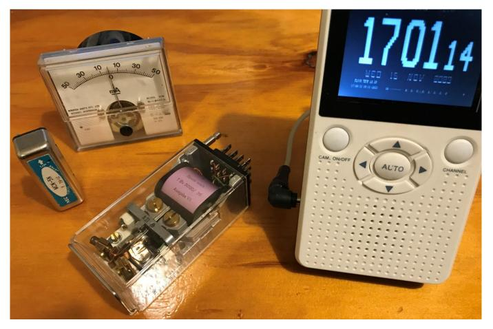
Some TTY trinkets along with the 2.4GHz receiver mentioned above. The panel meter is from Telstra TSG, used to monitor Telex signals while testing and repairing Telex machines. The smaller relay is Mercury wetted and must be used in that orientation, or it turns into a dead short as the mercury floods the contacts located at the top.
