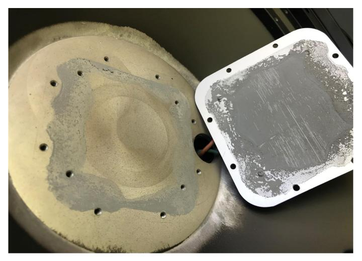
So I looked further and was shocked by how badly the LED module had been thermally bonded onto the heatsink, it was only making contact on the edges, the centre of the module does have thermal paste, however you can still see the original brush/applicator strokes, that part, where most of the LED's reside never made contact with the heatsink. It's amazing it lasted as long as it did. Now check out those LED's, boy have they been baked.
