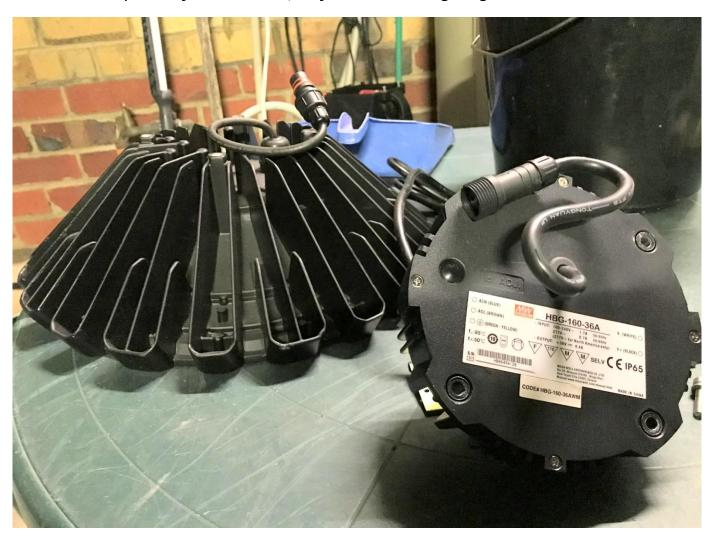
There is actually a plug and socket, nice. However no sign of any feedback for LED derating.
