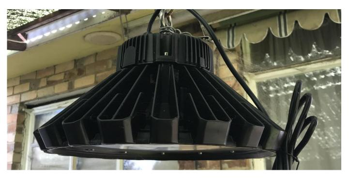
This is a more or less side view, they come it two pieces, you can probably spot the socket screw holding the upper power supply to the bottom lamp & reflector assembly
