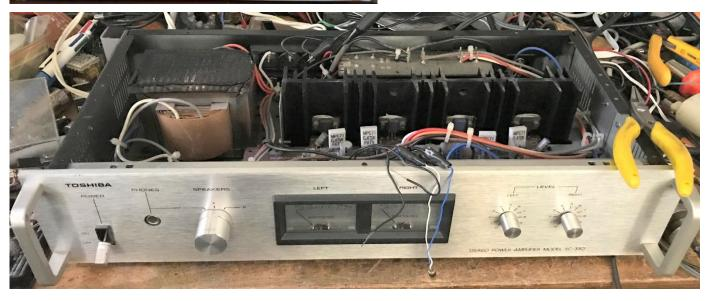
It cleaned up really well, the faults were a blown output fuse on one channel, very scratchy pots and two blown dial lights.
