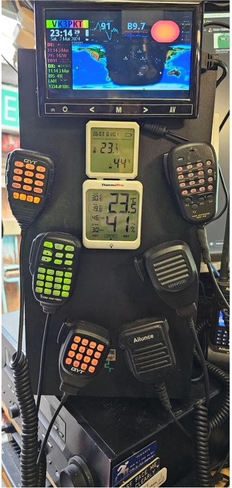
This is how I "Mount" my microphones. I superglue or screw on neodymium magnets to the back of the mic and the front of my PC tower is steel, the mics hold on well. There are 5 FM rigs in the shack and one mic is for my DMR handheld that sits in its charger
