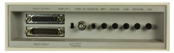
The KTX1350 has a composite video input connecter and can mix its own graphics with that and display in on the screen. As in overlay etc, it could not actually 'process' that video
