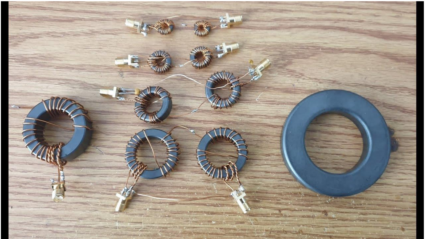
Antenna building #2 - EFHW Ant - figuring out the right core size https://youtu.be/nNzTf1F12BE
