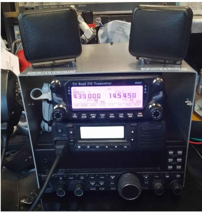
A stack of radios for Chris VK3VKK in a limited space environment there will be a short whip about 30-40 cm long that can handle 25watts that will go on the top of the aluminium case connected to the dual-band Zastone at the top of the stack.
