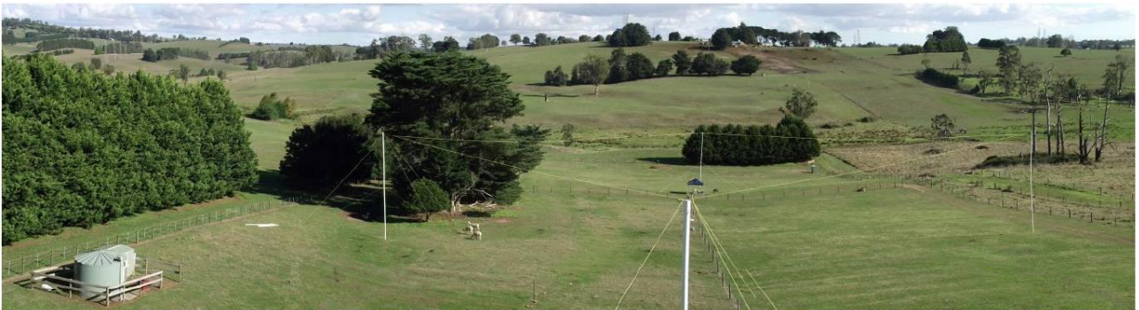
The completed 12 metre high rhombic antenna on 40 metres. (wire radiator enhanced for clarity)
