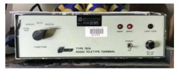
To make it compatible with a radio, as in Radio TTY, or RTTY, you need to convert it to audio tones that can be fed into a microphone socket, using something like this Codan box, although some radio's do allow you to feed serial data straight in and the radio will do the rest – I've
