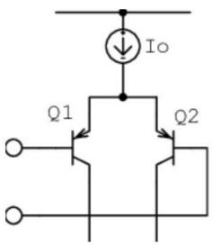
One transistor gets the incoming audio, whilst the other is fed from the amplifiers output, basically trying to correct the non-linearity of it to give us way lower distortion.
