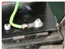
On opening it up it was pretty clean inside, and a quick electrical check only showed a bad mains earth connecting, so I made that my first task. Usually one connects the mains earth wire to the chassis using an unpainted area, for good electrical connection, something Eminar neglected to do, so the earth lug was nicely riveted to the chassis, but with a few mega ohms of resistance.... Not good. So I drilled out the rivet, ground back the paint then fitted a few serrated washers and a socket
