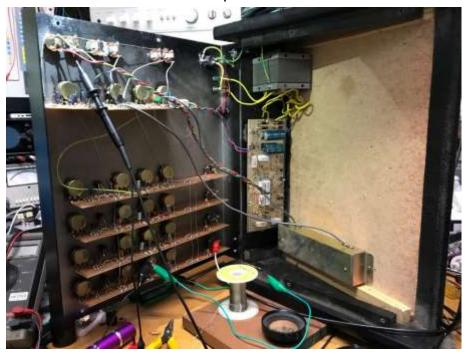
So now it was time to feed in some 400Hz audio tone and start chasing it through the system. I got slightly side tracked on the mixer strips as the audio was very distorted, but I then realised that if this was the fault I'd have a badly distorted output. Hower this was not the case, I was just expecting those mixer strips to put out way more than they did, and the the fault actually resides in the power amp at the back. I was simply over driving them. Usually an op-
