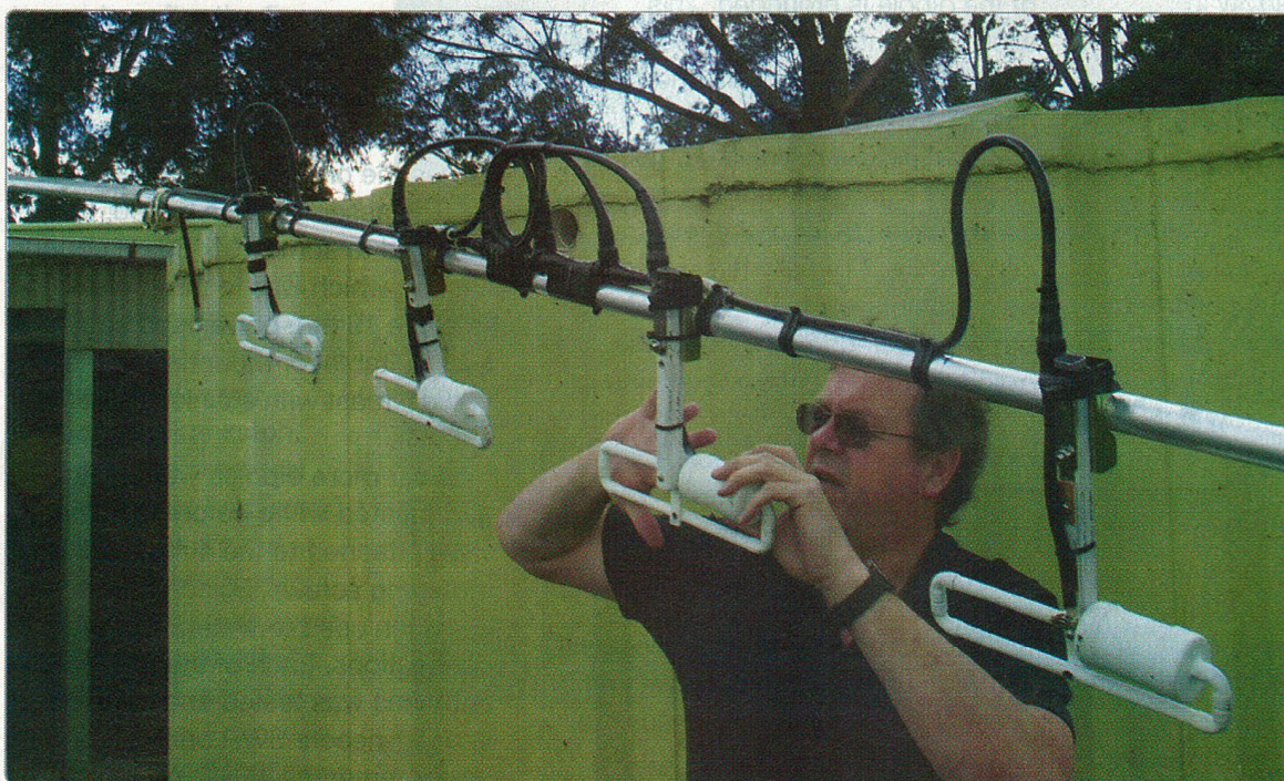
Photo 5: Rob VK3BRS waterproofing the tuned antennas.
