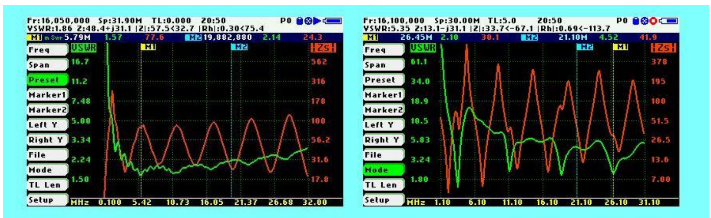
Left – the flat HF response of the Rhombic.
